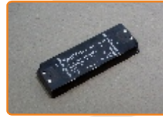
LED power supply 50W • Pri: 200-240V-50/60Hz • Sec: 12V DC eff, 4.17A • max load 50W • short circuit protection 15650000
