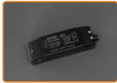
LED power supply 10W • Pri: 220-240V-50/60Hz • Sec: 12V DC eff, 800mA • max load 10W • short circuit protection KLP-1018HV
