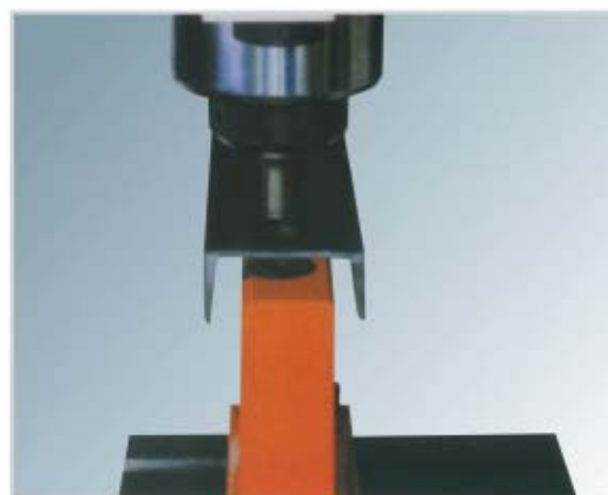
槽钢正面冲孔模具 Single hole die holder for punching channel webs.(optional on double cylinder models)
