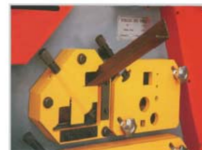
角钢剪断和45° 剪切, 四面刃口都可以调换 Single shear with no material loss and minimum deformation 45° miter-cut is easy and clean featuring blades with four usable cutting edges
