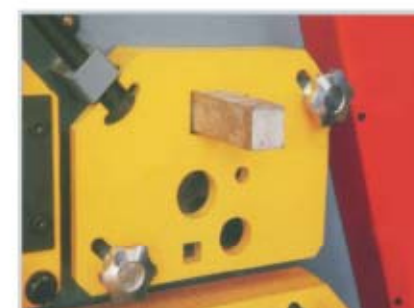
圆钢、方钢、槽钢、I字钢剪断 Round and Square bar shear with multiple holesfor variety of Sizes Adjustable hold down for clean square cutting,Optional Channel and Joist shear.
