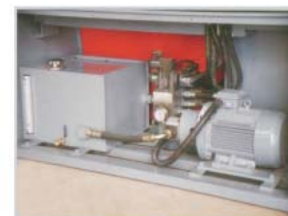
高品质的马达和通用的内置滤油器使保养更为简便 Quality high horse powermotors, with universal oil filter for ease of maintenance
